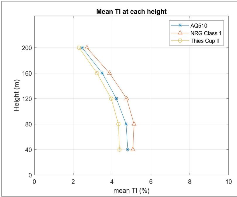
The AQ510 performs well in measuring mean TI over the period, standing always between the NRG Class 1 and Thies Cup II
