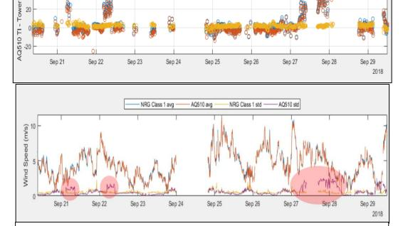
Examination of the time series (individual 10-minute points) showed that differences in standard deviations, rather than differences in wind speeds between the anemometer and the AQ510 had more effect on the calculated TI. It was noted in the investigation that this situation tended to occur at low wind speeds.
